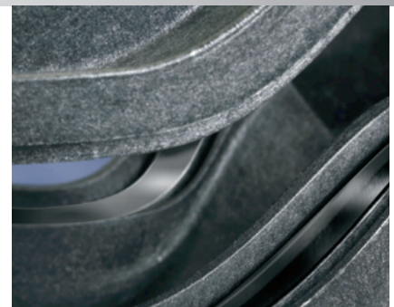
Close-up of under-the-hood part showing molten edge ready to be sealed.
