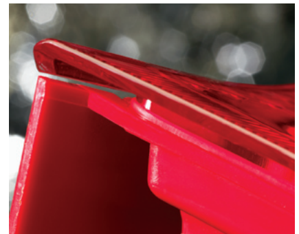
Preheating allows delay of vibration until the viscous stage, avoiding the particulates that result from friction of dry solid-solid vibration.
